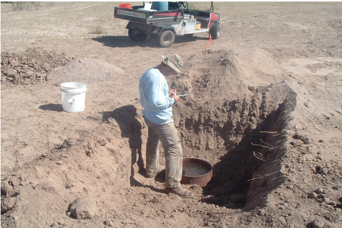
Figure 4-12. Cylinder Infiltrometer Test at Depth
